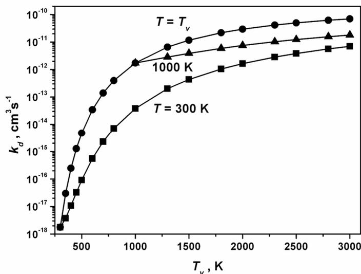
Fig. 1: The detachment rate constant as a function of vibrational temperature of  $\text{O}_2$  for  $T = 300$  and  $1000$  K and for  $T = T_v$ .
