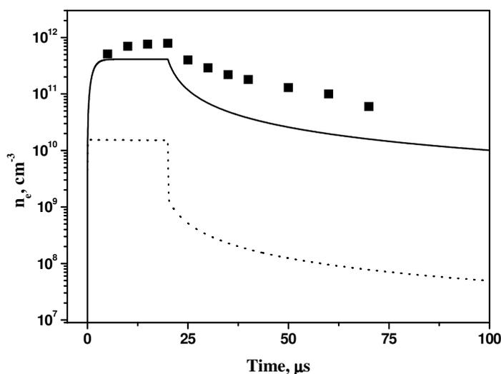
Fig. 2: The evolution in time of the electron density in atmospheric-pressure air plasma generated by an electron beam of duration 20  $\mu\text{s}$ . Solid curve corresponds to  $T_v = 2500$  K,  $T_e = 5000$  K and  $T = 560$  K and dotted curve corresponds to  $T_v = T_e = T = 300$  K. Symbols correspond to measurement [2].
