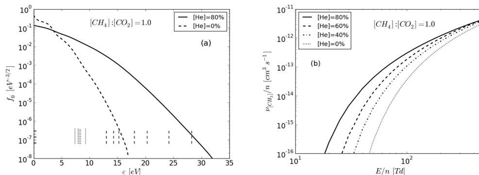
Fig. 1: Results in He/CH<sub>4</sub>/CO<sub>2</sub> mixtures: (a) Isotropic component of the electron energy distribution function at  $E/n = 50$  Td. Vertical lines: threshold values for vibrational excitation, dissociation, ionisation and attachment. (b) Variation of the density-normalized collision frequency for dissociation of CH<sub>4</sub> into CH<sub>3</sub>, with  $E/n$  for several helium concentrations.
