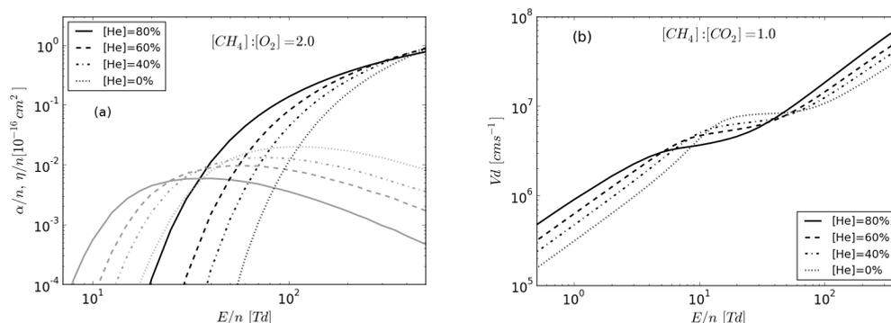
Fig. 2: Effect of helium concentration on (a) the density-normalized ionisation and attachment coefficients in He/CH<sub>4</sub>/O<sub>2</sub> mixtures at a constant ratio [CH<sub>4</sub>]:[O<sub>2</sub>] = 2.0 (black lines:  $\alpha/n$ ; gray lines:  $\eta/n$ ) and (b) the drift velocity in He/CH<sub>4</sub>/CO<sub>2</sub> mixtures at a constant ratio [CH<sub>4</sub>]:[CO<sub>2</sub>] = 1.0
