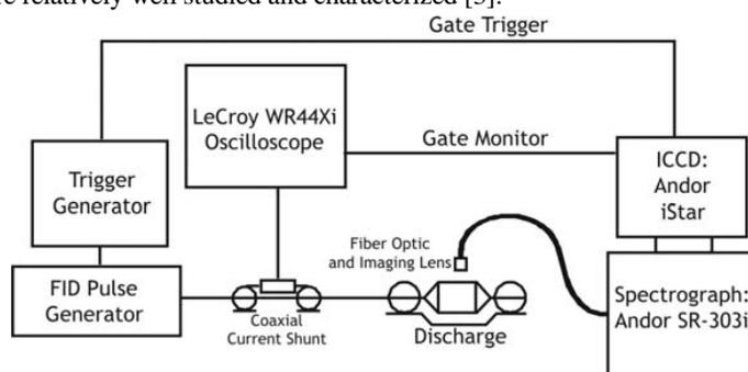
**Fig. 1** Scheme of the experimental setup for measurements of energy input and gas temperature.
