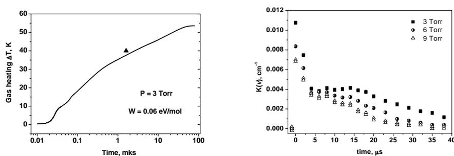
**Fig. 2** (a): calculations (curve) and experimental measurements (triangle) of temperature increase for similar FIW conditions in air; (b) CRDS measurements of  $\text{N}_2(\text{A}^3\Sigma_u^+)$  ( $v'=0-v''=2$ ) absorption in synthetic air in the FIW afterglow for different pressures.
