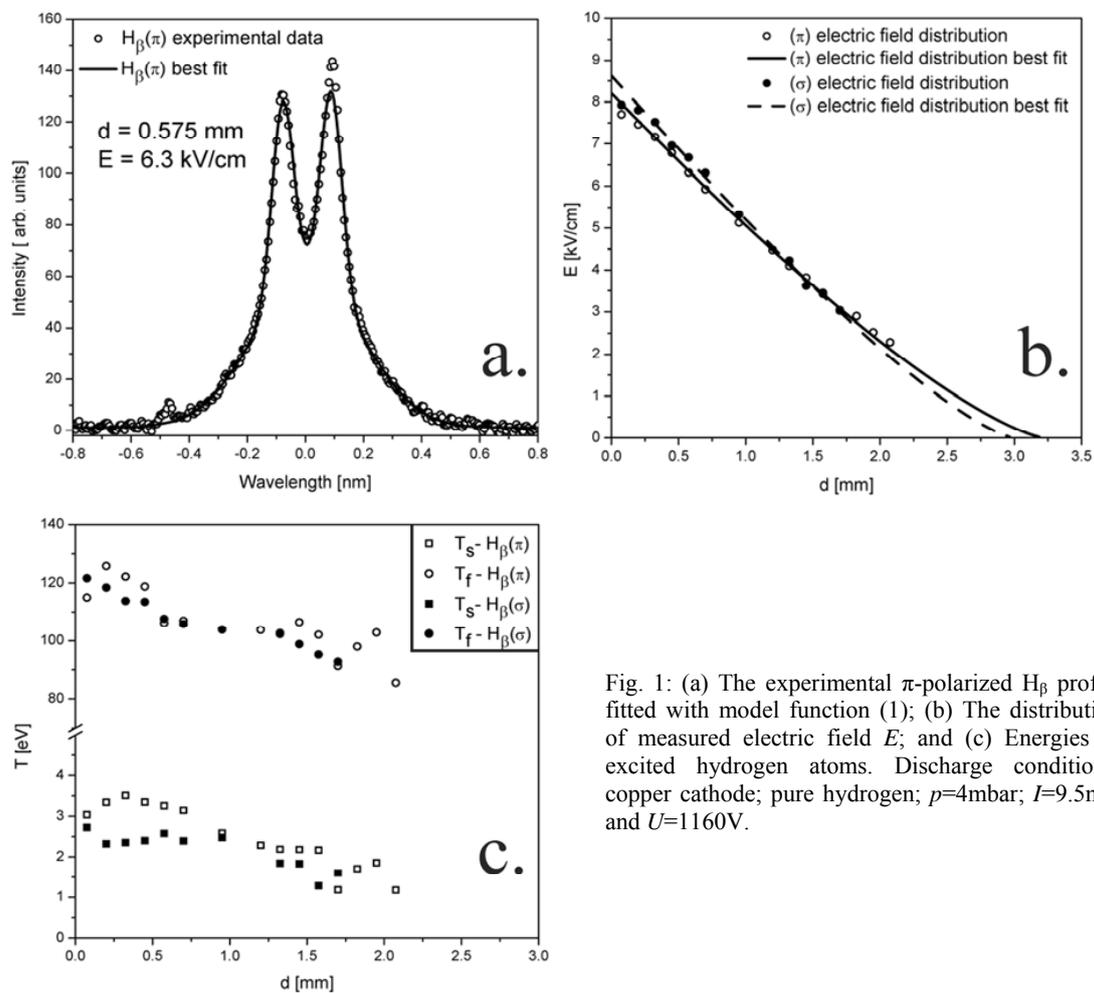
Fig. 1: (a) The experimental  $\pi$ -polarized  $H_{\beta}$  profile fitted with model function (1); (b) The distribution of measured electric field  $E$ ; and (c) Energies of excited hydrogen atoms. Discharge conditions: copper cathode; pure hydrogen;  $p=4$ mbar;  $I=9.5$ mA and  $U=1160$ V.
