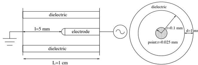
Fig. 1: Sideview and topview schematics of discharge set-up.
