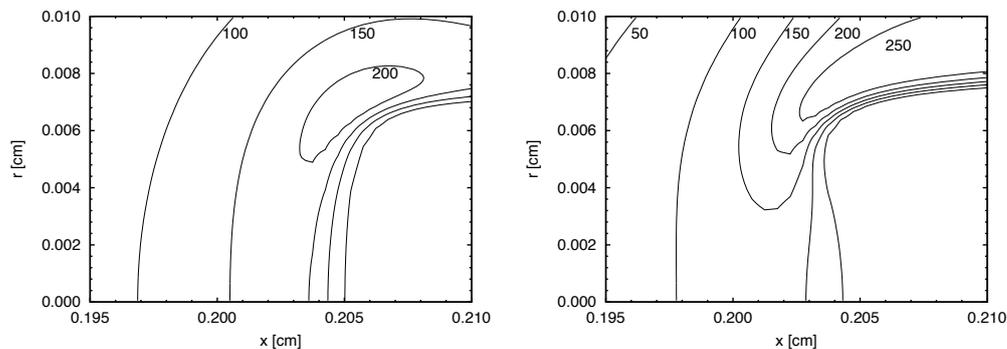
Fig. 2: Isocontours of total electric field when the discharge is at 0.2 cm from the cathode. Applied voltage: 6 kV, left figure:  $\epsilon = 1$ , right figure:  $\epsilon = 5$ . Contours vary from 50 kV/cm to 250 kV/cm.
