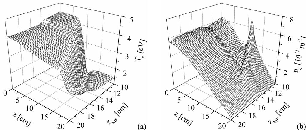
Fig. 2: Axial variation (at  $x = 0$ ) of the electron temperature (a) and density (b) for different positions  $z_{MF}$  of the magnetic filter; gas pressure  $p = 8$  mTorr and magnetic induction  $B_0 = 50$  G at its maximum.
