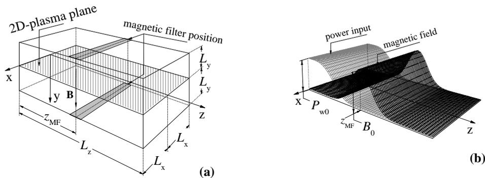
Fig. 1: Configuration and dimensions ( $2L_x = L_z = 20$  cm) of the discharge vessel (a) and axial variation of the filter field and of the power deposition to the discharge (b).
