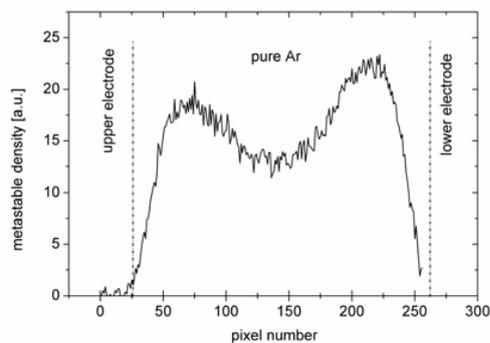
Fig. 2. Spatial Ar\* density distribution in a pure argon discharge.
