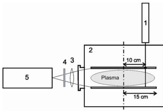
Fig. 1. Experimental set-up, side view: 1- Laser diode 772.38 nm; 2 - plasma chamber; 3 - objective; 4. interference filter at 810 nm; 5- CCD camera.
