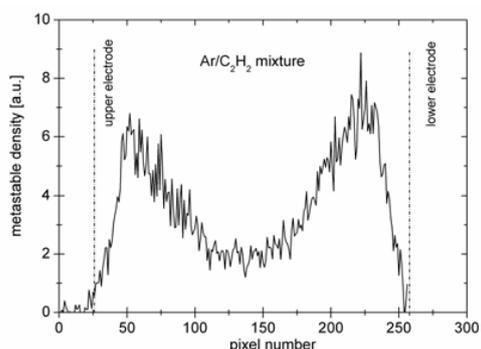
Fig. 3. Ar\* metastable density distribution in Ar/C<sub>2</sub>H<sub>2</sub> discharge, before dust particles formation.
