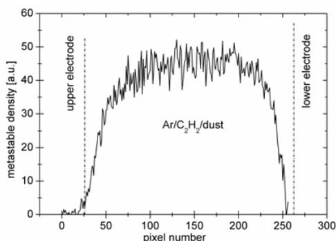
Fig. 3. Ar\* metastable density distribution in Ar/C<sub>2</sub>H<sub>2</sub> discharge after dust particles formation.
