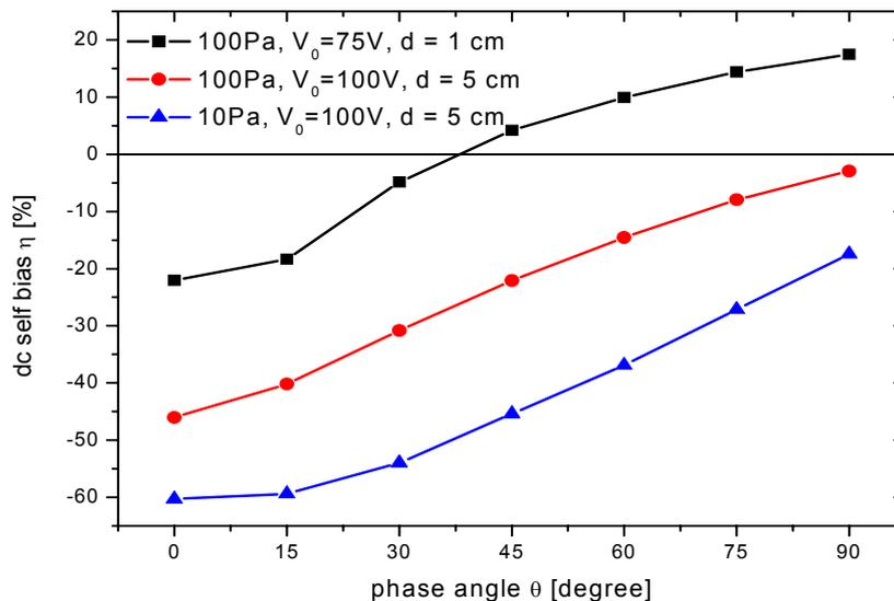
Fig. 1: DC self bias  $\eta$  (normalized to the applied voltage amplitude) as a function of the phase angle  $\theta$  between the driving frequencies for different chamber geometries (squares: plasma confinement by a glass cylinder, 1 cm electrode gap / circles and triangles: plasma confinement by a metal mesh, 5 cm electrode gap).
