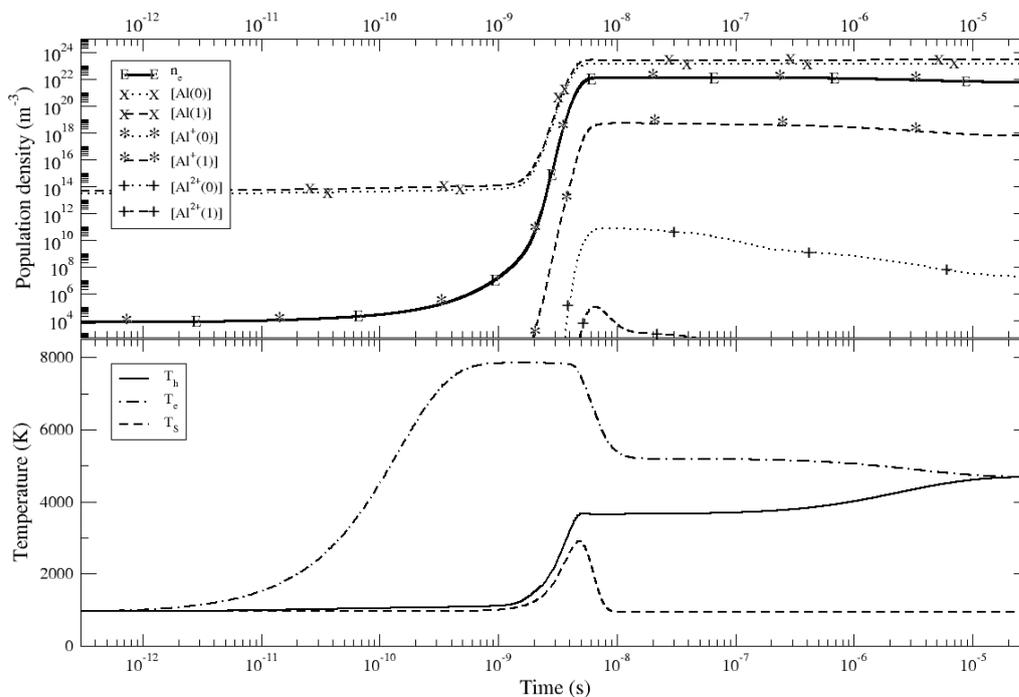
Fig. 1: Population density (up) and temperatures (down) of plasma components calculated by the CR model A.
