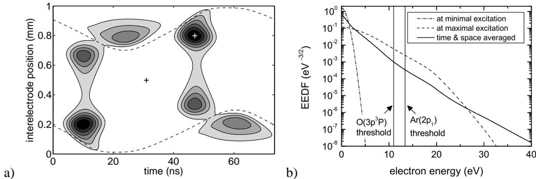
Fig. 2: a) Simulated time and space resolved electron-impact excitation rate coefficient for the Ar(2p<sub>1</sub>) state on a linear gray scale starting from zero. The dashed curves indicate the sheath edges. b) Calculated EEDF. Time and space of minimal and maximal excitation is marked in subfigure a) by crosses.
