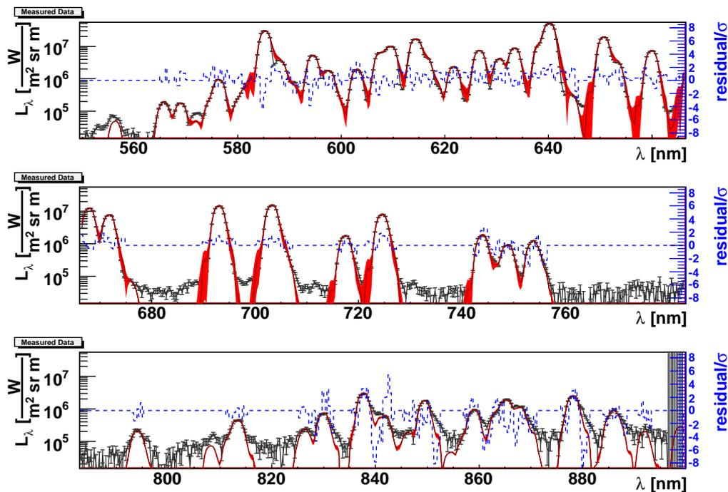
Fig. 2: Intensity of light emitted from a neon discharge as a function of wavelength. The light-colored (red) curve depicts the modeled spectrum, including the uncertainty of the apparatus function. The measured spectrum with the experimental error bars is partly hidden behind the modeled spectrum. The dashed (blue) line represents the difference between model and measurement in units of standard deviations. For details, see [19].
